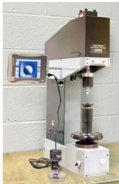
Shown: The PB7100 tester with B.O.S.S. Brinell optical scanning system.
