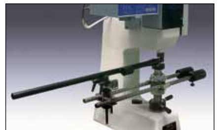
A range of accessories are available for testing difficult shapes. Seen above a unit is testing a gun barrel using a counter-balanced jack rest and gooseneck adapter.
