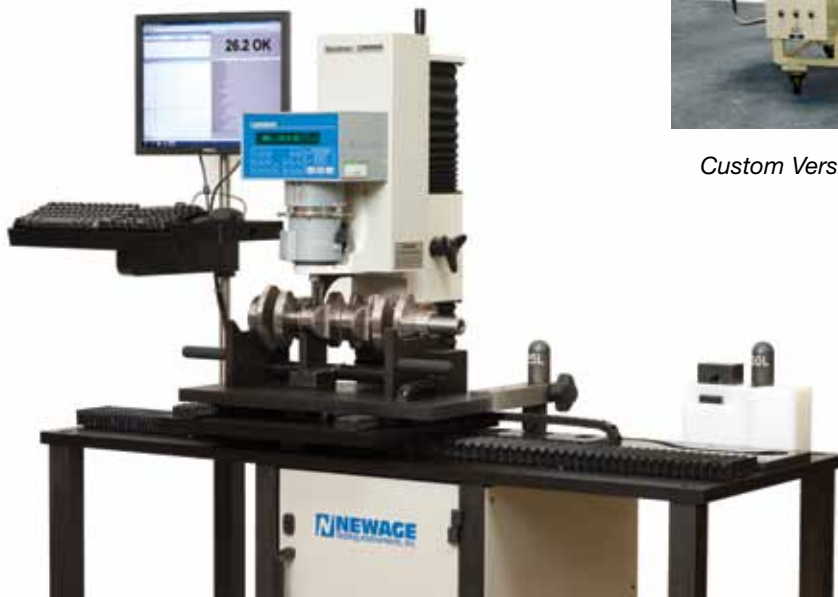
Custom Versitron® Test System for automotive crankshafts.
