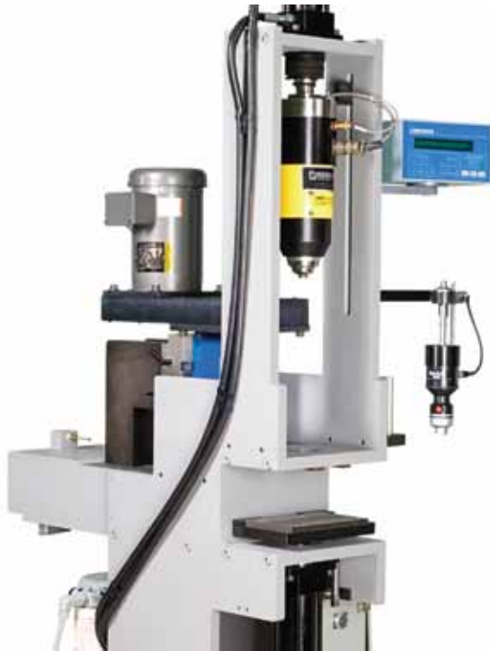
Custom Automatic Brinell with depth & optical measurement and automatic surface preparation.
