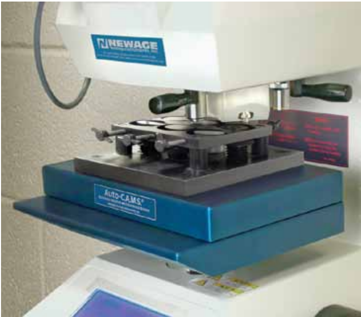
(Above) The motorized positioning tables are built specifically for hardness testing using optical encoders with 0.5 micron resolution. In addition to the fine positioning over long ranges, the optical encoders enable a positioning system that is much less subject to positioning error due to frictional wear on the screws - a factor which is accentuated in heavier multi-sample systems.
