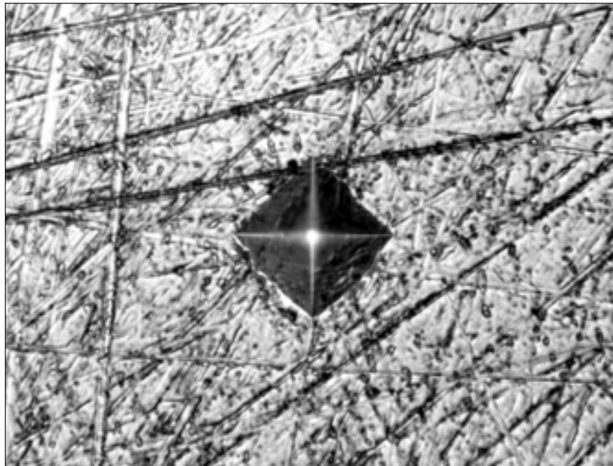
A Vickers indentation, as it appears on a rougher ground surface, showing potential for tip identification problems from grind marks
