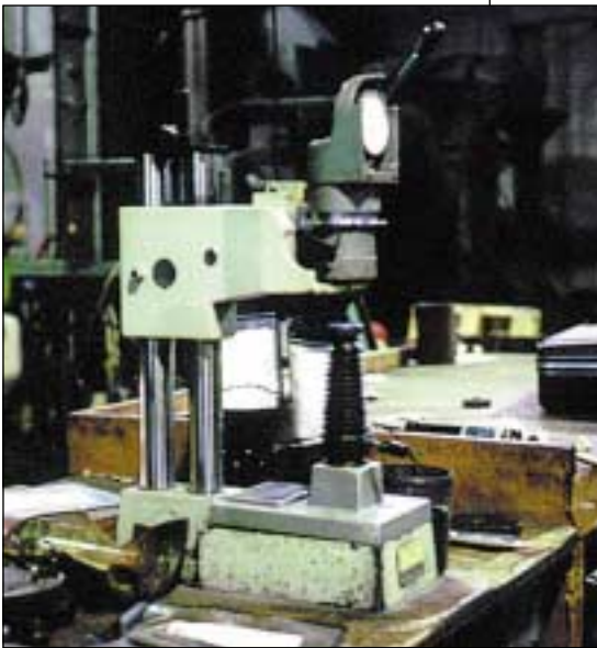
Fig. 3 — Rockwell hardness testers are often asked to perform in harsh environments. In these cases, says the author, the elevating screw and its bearings should be cleaned during every servicing of the instrument.
