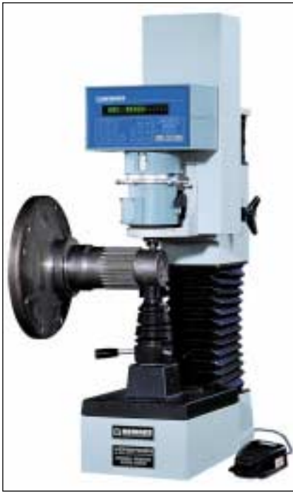
Fig. 2 — Proper support of parts is critical. Some machines, such as this one, are capable of clamping parts prior to the application of loads, providing a stable test piece.
